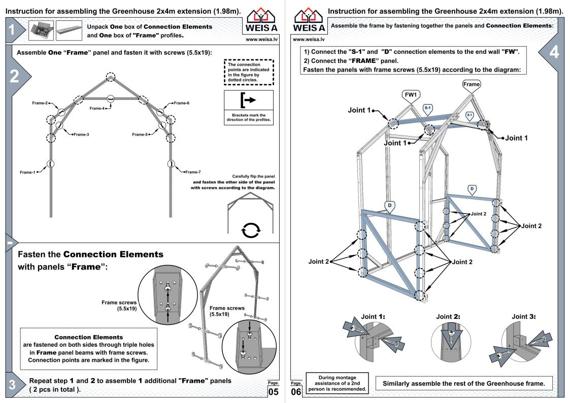
Instruction for assembling the Greenhouse 2x4m extension (1.98m).
